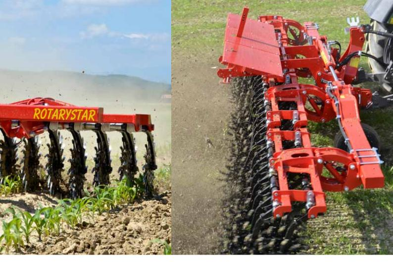
Via a hydraulic parallelogram the pressure on the sections can be adjusted during operation. In addition this system allows to control the level of the rotor section and distributes the pressure in between the sections in uneven terrain.
