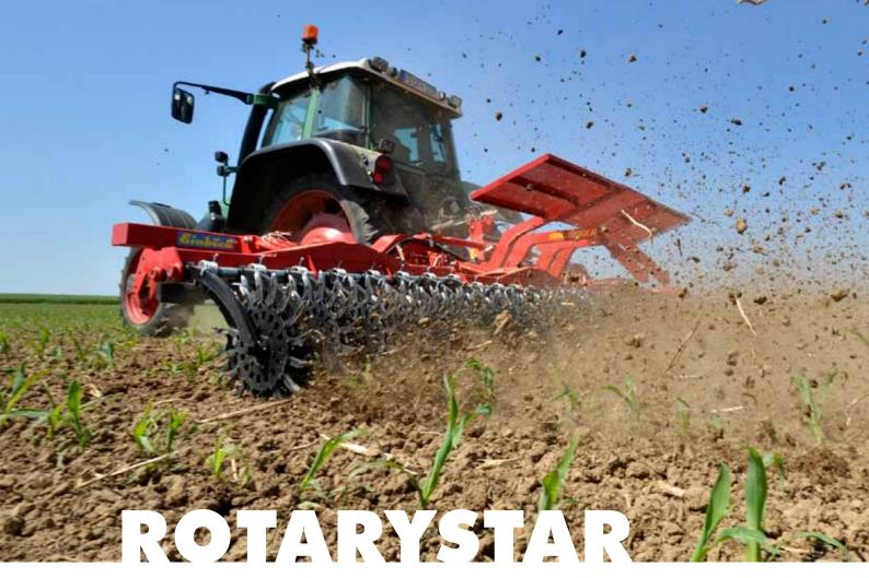
Due the rolling motion of the rotor stars no plant residues are collected – ideal to fight weeds in mulch-till crops.
